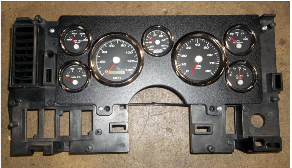
FIG 3: CLUSTER INSTALLED IN STOCK CARRIER WITH 4 EA #8X1" SCREWS
