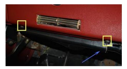
Remove the screw for the air duct (yellow) and drop the duct.
