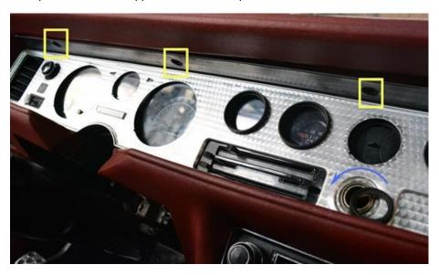
Remove the 6 screws that hold in the 2 piece gauge clusters. Pull out the gauges, remove the wiring plugs, speedometer cable, etc.
