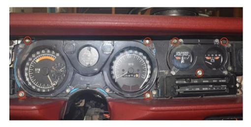
Installation is the reverse of removal. Use the standard hardware that was removed to re-install the panel.
