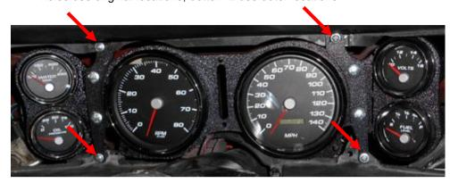
Install OE bezel. Note location of gauges in relation to the openings. All instruments can be adjusted via the slotted bracket openings. Outer gauge fore/aft can be achieved with  $\frac{1}{4}$ " spacers included in package. If needed entire bracket can be brought rearward in vehicle by swapping the mounting brackets to the back.
