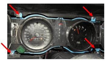
Test fit cluster in dash, attach using original fasteners. Top 2 holes use original locations, bottom 2 use outer locations
